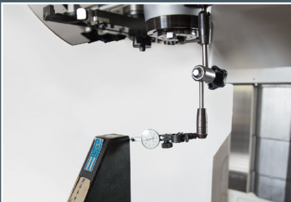
Y, Z axis vertical adjustment
