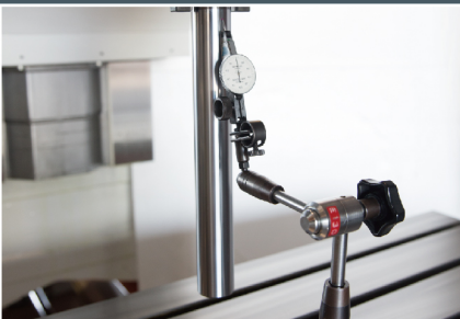
Spindle run out inspection test
